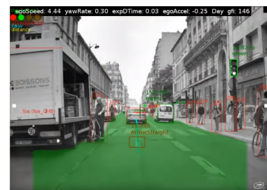
Mobileye uses computer vision algorithms to detect free road space, traffic signals, signage, vehicles, and pedestrians.
